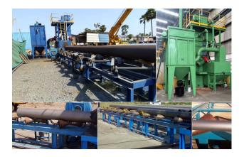
Diablo type rollers and tire type conveyor are used to convey Pipe for automatic shot blasting process. Machine can be designed for pipe ranging from 1/2 " to 60" dia and normally supplied with Feeding, buffer stock, loading & unloading systems. Very commonly used in pipe coating industry, pipe lines projects in petroleum, power, oil & gas, petrochemicals industries. Machine can be designed of the size & design of fright container which can be used for cross country pipe line projects.
