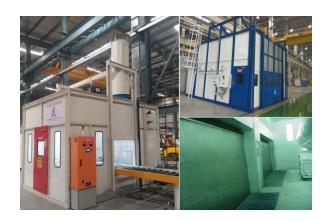
Wet type paint booths supplied with water curtian system, water scrubber system and with full water floor system.
