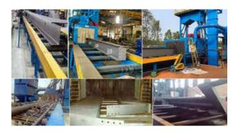
These type of machines are widely used in automobile & steel fabrication industry. Fabricated structure, Chassis of vehicles, panels of tippers and trailers etc. are shot blasted on SKD form on these machines. Turbines are designed and located in such way that the job is shot blasted from all angles. Machine are available of sizes ranging from 2.5 meter x 0.5 meter opening to 3.5 meter x 2 meter opening.
