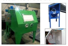
Suction cabinets are for very small jobs and for laboratory purpose. Cabinet is provided with hand gun for small area blasting.
