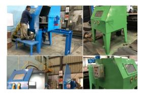
Pressure blast cabinets are for small components blasting. It's a portable equipment with in built pressure blaster, nozzle and with dust collector. Can be supplied with turn table, trolley for job handling.
